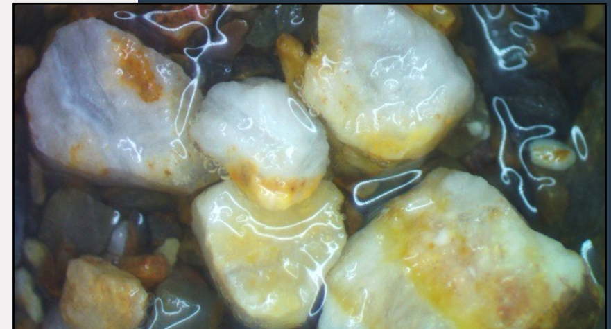
Binocular microscope photo of Interval 134.1–135.6m from LSRC04 assayed 9.6 g/t Au, 122.2 g/t Ag showing oxide
